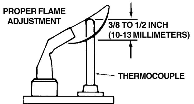
**Figure 11. Proper Flame Adjustment**
